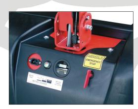
Built-in high Frequency batteries charger
