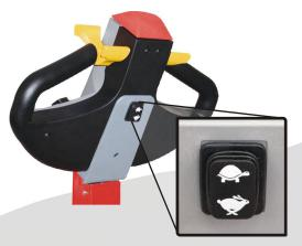
Speed Selector to operate with the tiller in the upright position
